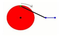
A rod is connected to a rotational crank, by moving the rod a circular motion is created. Alternatively, turning the rotational crank creates a linear motion.
